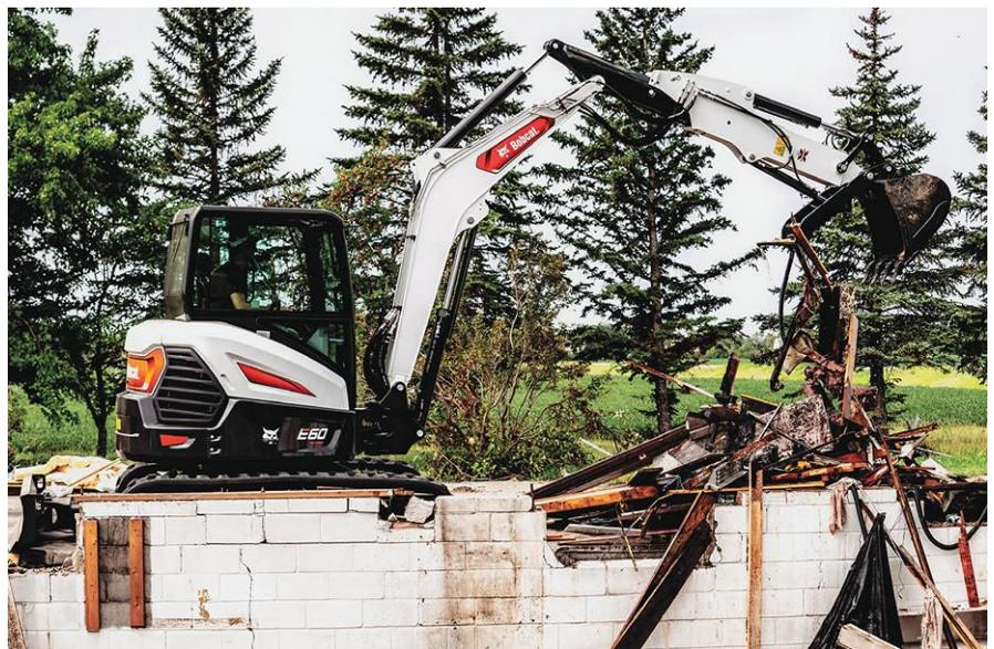
demands different features. If you work in confined areas like residential properties or commercial jobsites, every inch matters. Larger excavators can weigh more than 10 tons, so make sure your jobsite can accommodate the overall size and weight of a larger machine.
